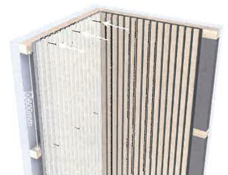
c. Install fibreglass wool or rock wool between the battens. absorption class: A
