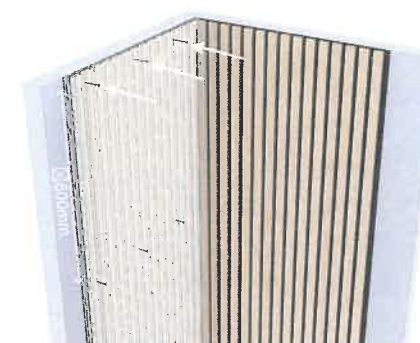
a. Nail acoustic panels directly to the wall. absorption class: D
